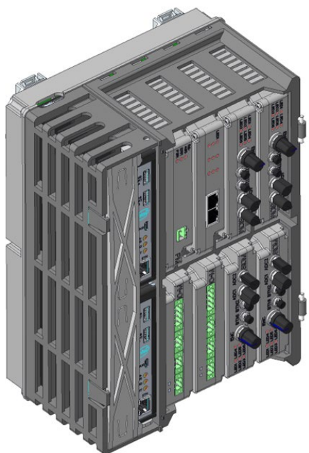
Figure 2: A rendering of a modular E4S platform, based on the E4S Alliance’s requirements. The dimensions are 280mm x 150mm x 205mm. Image from Delta Electronics, Inc.
